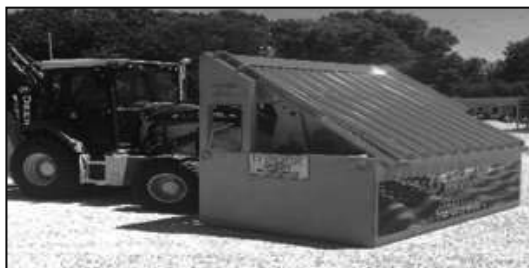
MR10 Model , 1-2 yd loaders. Adjustable bar and Cleaner option available. Removable cleaner for more sorting options
